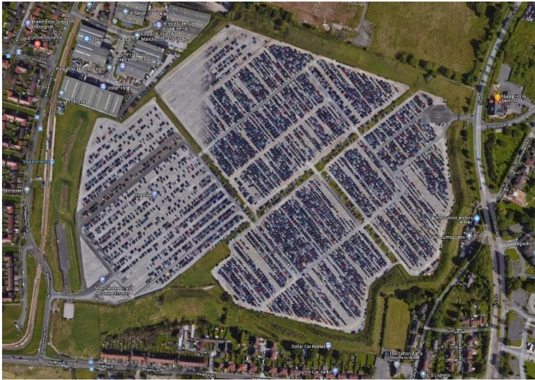
Figure 4-9. Example of block parking at Manchester Airport, UK
